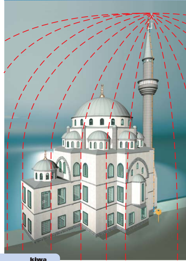
Protection zone provided by a FOREND ESE rod
